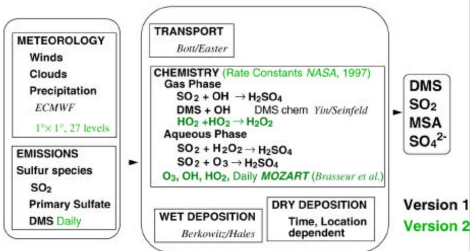
Figure 1. Key elements of the aerosol chemical transport model. Extensions beyond the original model are indicated in green (Version 2).
